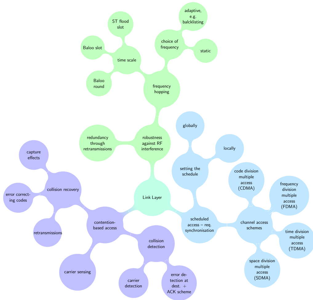
Figure 2.5: Overview of link layer techniques useful in wireless collection scenarios.
