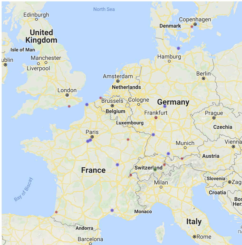
Figure 4.3: 10 most important hubs computed on the Western Europe graph. Blue dots mark the time graph hubs, red dots the distance graph hubs and green dots hubs that coincide between the two graphs (only Gotthard Pass).
