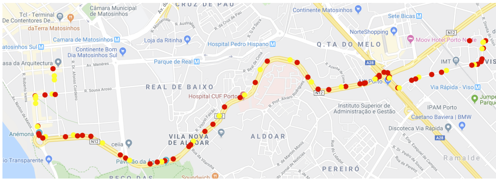
Figure 3.2: GPS trace and its matched path. Yellow dots mark the raw GPS trace, red dots mark vertices along the matched path.
