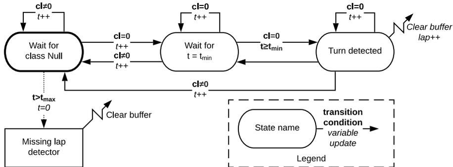
Figure 3.3: Finite State Machine for Lap Detection
