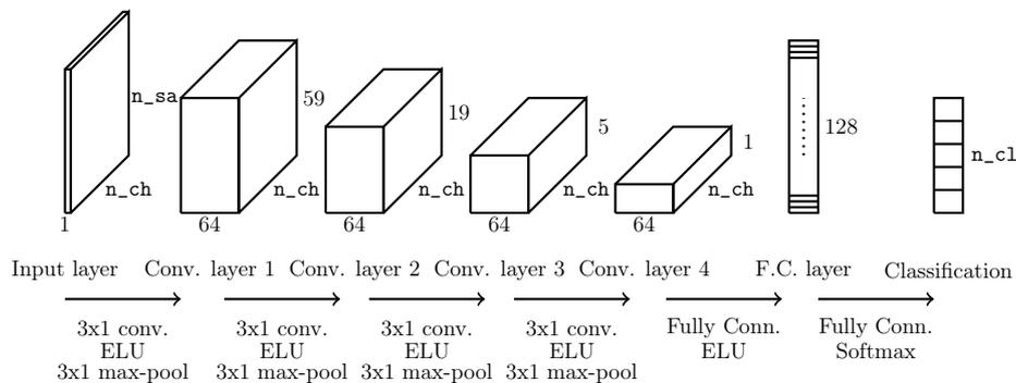
Figure 2.1: Structure of the CNN used for recognition [1]
