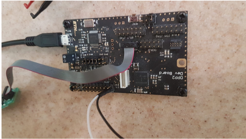
Figure B.8: setup, zoom into logic output's connection with the RocketLogger
