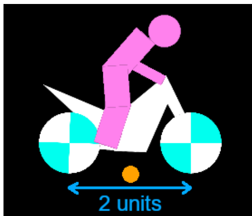
Figure 2.5: Screenshot of the motorbike at rest with a scale reference. Its position \mathbf{b} is given by the position of the orange dot. The angle of the bike is \theta = 0 .
