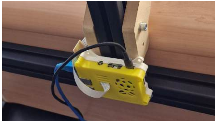
Figure 2.9: Raspberry Pi 5 (with lan-cable, power-cable and csi-cable) mounted to the aluminium extrusions
