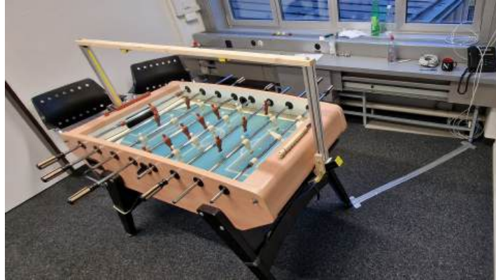
Figure 3.1: Cameramount installed onto the foosballtable
