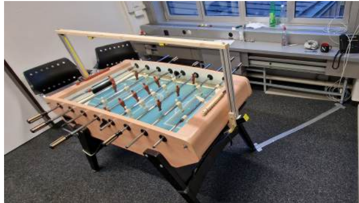
Figure 2.10: Foosballtable with installed cameramount, raspberry pi are installed onto the aluminium extrusions and all the cables (one powercable, two ethernet cables) are properly taped to the ground
