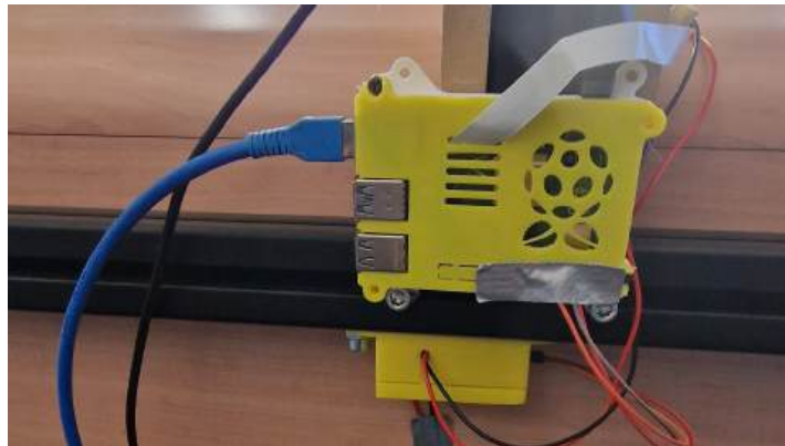
Figure 2.8: Raspberry Pi 5 connected with 3 cables to the relay (yellow box below) which will control the led strip
