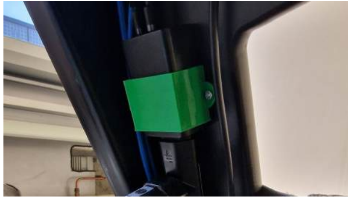
Figure 2.6: Powersupply for the raspberry pis (65W), mounted with the help of a 3d printed holder to the leg of the foosballtable
