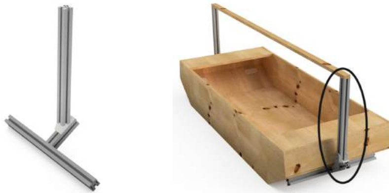
Figure A.4: Aluminium extrusions overview, and where they are located on the foosballtable
