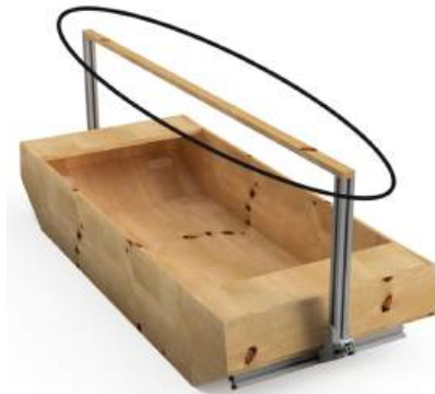
Figure A.11: The wooden strip is mounted on top of the aluminium frame.
