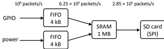
Figure 4. Data flow and memory structure of the data acquisition system. The SRAM serves as buffer for the SPI bus. The two data streams are merged when writing to the SRAM.
