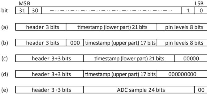
Figure 3. Data format of GPIO tracing and power profiling packets. All packets have a width of 32 bits and include a header of 3 bits. *Marker packets* (b) and (d) contain the upper 17 bits of the timestamp.
