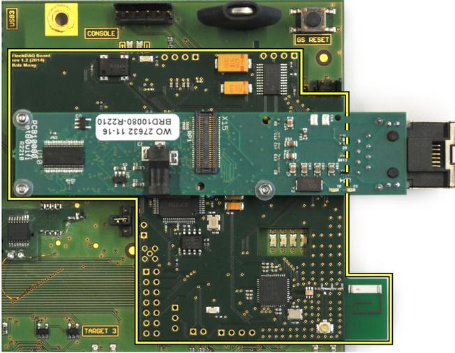
Figure 6. The TRACELAB board fits between the FlockLab board and the Gumstix. Visible on the lower right part is the CC430 with a chip antenna. The FPGA and the SRAM chip are on the bottom layer.
