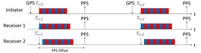
Figure 5. Generation of a synchronized 1-PPS signal. An external GPS pulse triggers the start of a flood at the initiator. The 1-PPS pulse is then emitted on all the nodes in the network based on the calculated reference time  $T_{ref}$ . This process is repeated every second.
