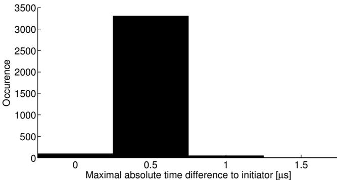
Figure 10. Absolute time synchronization error of TRACELAB. The histogram shows the maximal error of 5 out of 31 observers, relative to the root observer.
