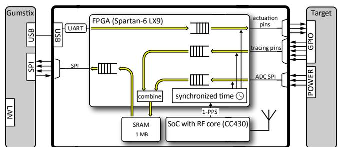
Figure 1. Overview of a single TRACELAB observer.
