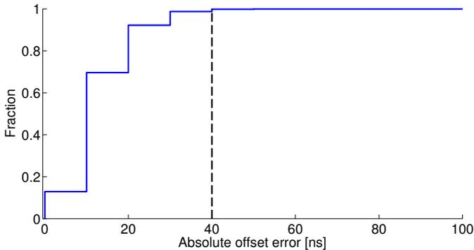
Figure 7. Cumulative distribution function of the absolute offset error between the internal and external 1-PPS signal. The clock tracking algorithm keeps the offset error within  $\pm 40$  ns for 99 % of the time.
