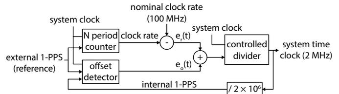
Figure 2. The clock control algorithm is a combination of an open-loop controller and a feedback control loop. The speed of the system time clock is controlled by a variable divider.
