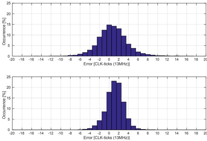
Figure 9. Distribution of synchronization error on node 4. The error distribution for the baseline implementation (top) is significantly broader than for the jitter reduced version (bottom).
