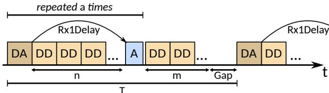
Figure 5. TDMA scheme with interleaved acknowledgment/sync packets.
