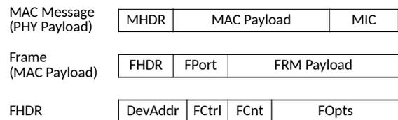
Figure 1. Frame structure of a MAC layer message.
