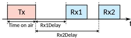
Figure 2. In LoRaWAN Class A end-devices only listen for packets during the defined receive windows.
