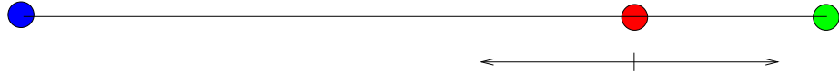
Figure 4.4: The testbed settings of the interceptor measurements. The blue node is the receiver, the green one is the sender and the red one the interceptor. The distance between the sender and the receiver is five meters and the position of the interceptor is variable.
