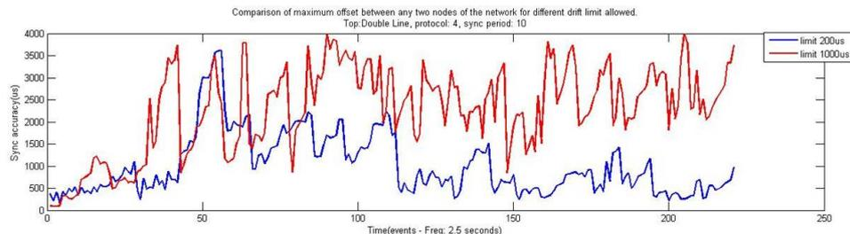
Figure 4.30: Impact of offset limit configuration.
