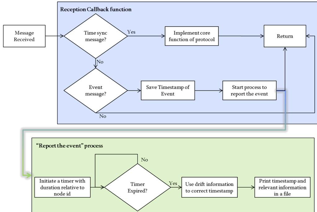
Figure 4.15: Timestamp and report of the event. The “report the event” process is called and runs in parallel to the protocol’s functions.
