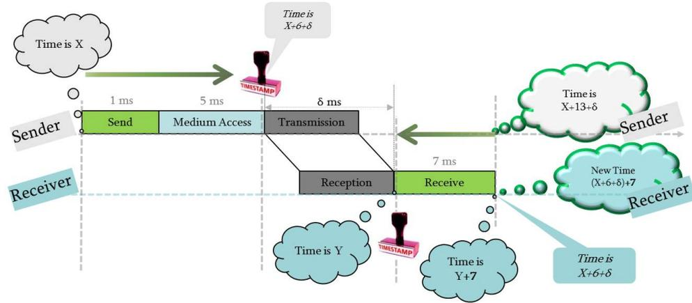
Figure 4.24: Timestamps at the MAC layer reduce the variance of the delay per hop.
