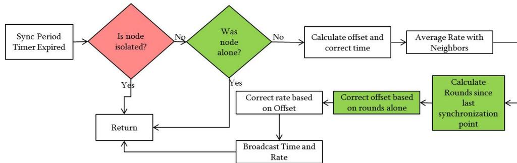
Figure 4.28: GTSP tracking the rounds that the node was alone.
