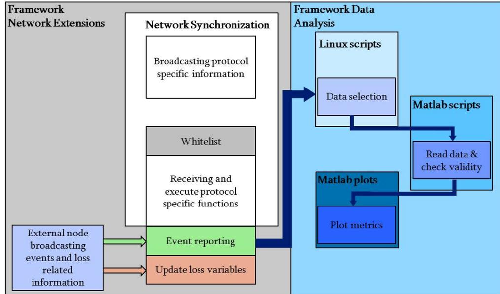
Figure 4.1: Evaluation framework: Its components and their integration.
