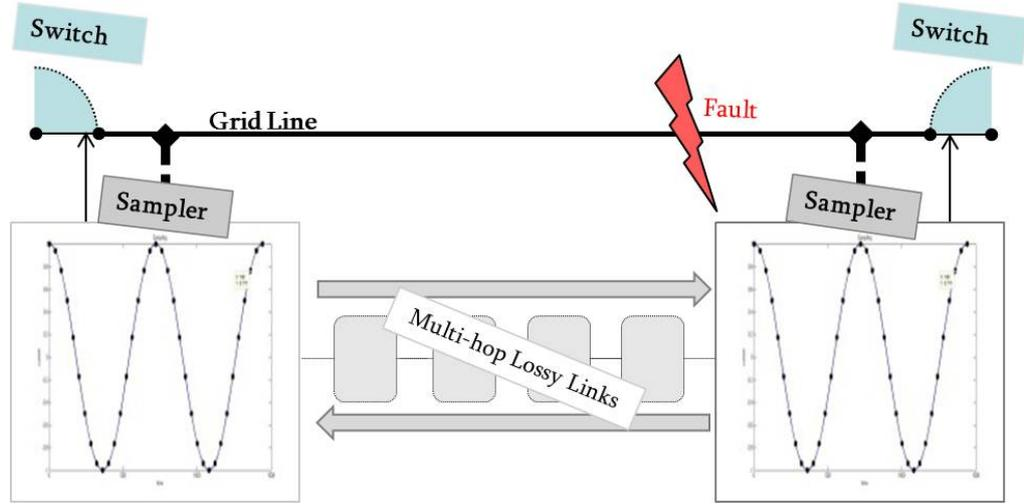
Figure 1.1: Grid line fault detection utilizing time synchronized samplers exchanging information over a multi-hop lossy network.
