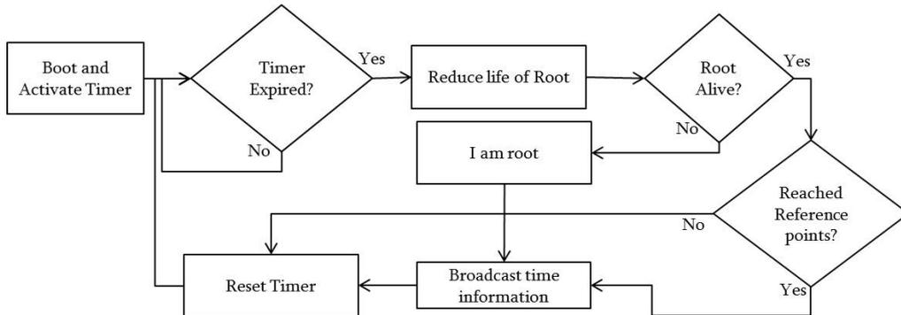
Figure 4.12: FTSP function when a synchronization period is over.
