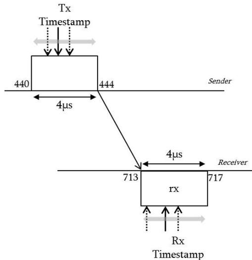
Figure 3.2: Example of error inserted by the limited timer resolution: The timestamp command can be issued at any time during the interval of  $4\mu\text{s}$ , leading to errors which limit the performance of time synchronization protocols.
