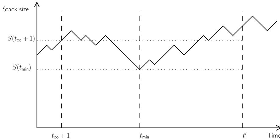
Figure 5.2: Lemma 5.4 is not fulfilled for  $t_{\infty} + 1$  and  $t'$ , because there exists a  $t_{\min}$  with a smaller stack size in between. The next iteration will check if Lemma 5.4 is fulfilled starting from  $t_{\min}$ .
