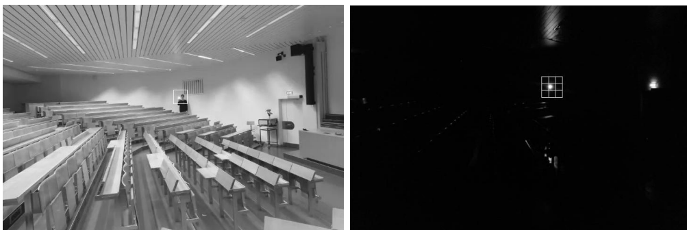
Figure 3.7: Blinking detection with the reflections on the ceiling removed.
