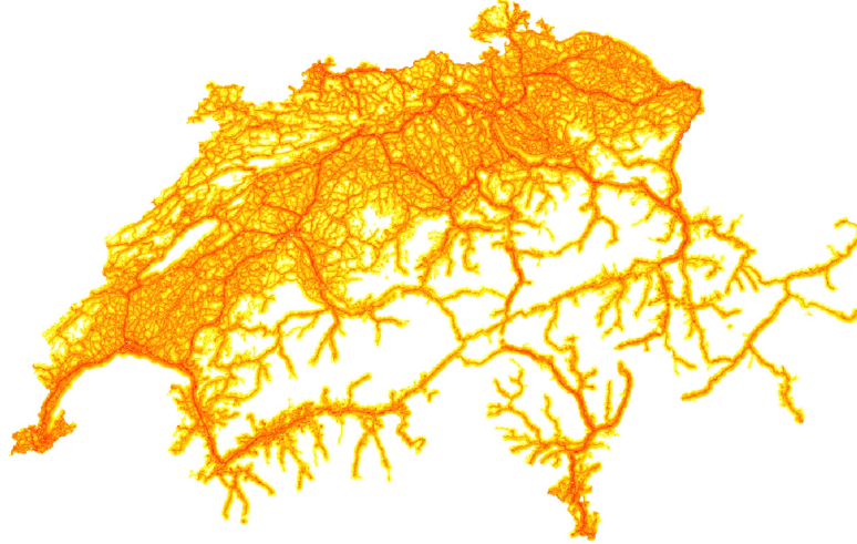
Figure 2.1: Road traffic noise model by day taking into account 72'000km of roads. Data resolution is a 30 m by 30 m and the data is given in decibel (red - noisy, light - quiet).
