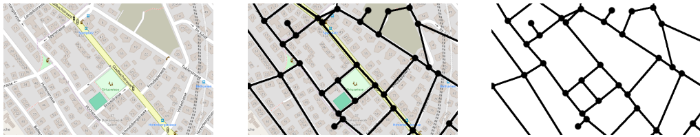
Figure 2.1: We convert the real world street network to a graph.
