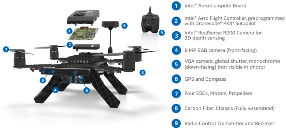
Figure 2.1: Intel Aero RTF drone [11]
