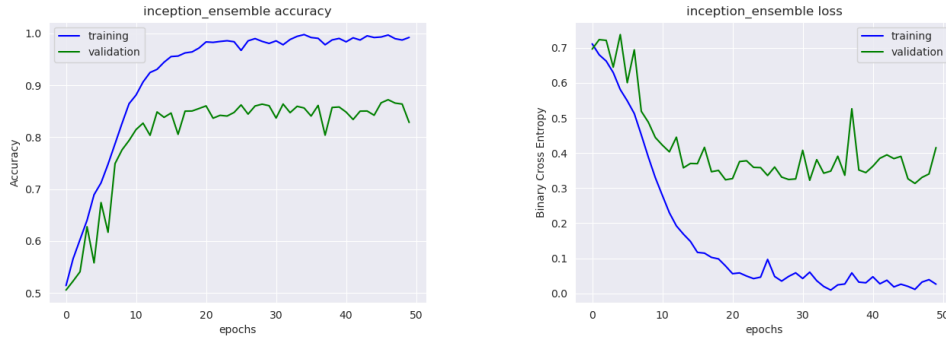
Figure 3.7: InceptionTime model with 20% training data and use_residual=True , kernel_size=40 , nb_filters=32 , depth=12 , bottleneck_size=16 , batch_size=64 .
