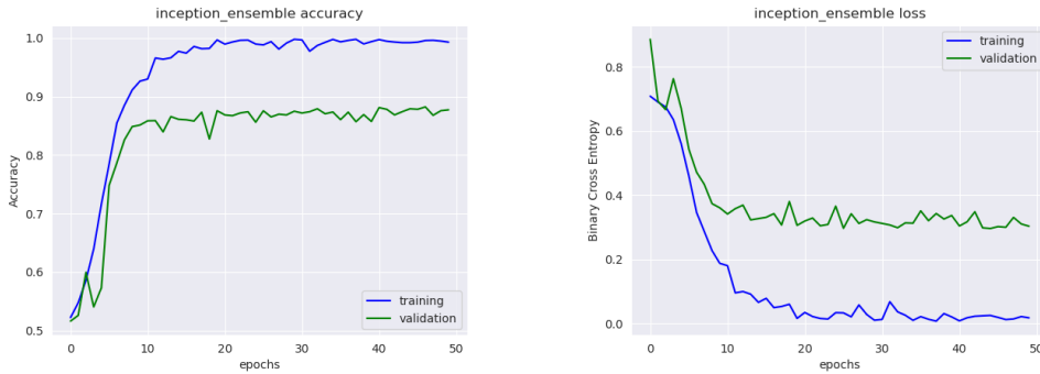
Figure 3.1: InceptionTime model with 20% training data and use_residual=True, kernel_size=40, nb_filters=32, depth=12, bottleneck_size=16, batch_size=64.
