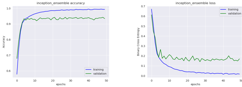
Figure 3.13: InceptionTime model with 100% training data and use_residual=True, kernel_size=64, nb_filters=16, depth=12, bottleneck_size=16, batch_size=64.
