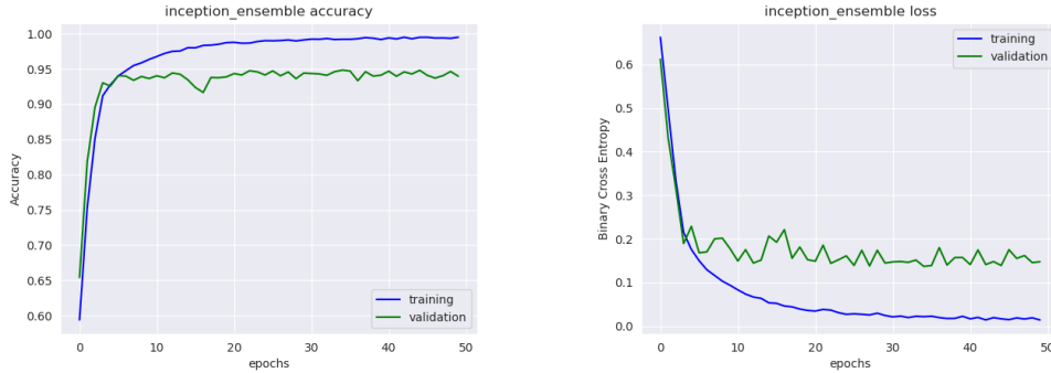
Figure 3.6: InceptionTime model with 100% training data and use_residual=True, kernel_size=64, nb_filters=16, depth=12, bottleneck_size=16, batch_size=64.
